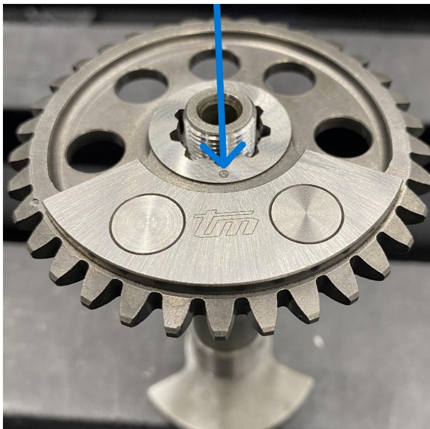
Figure 4: Balance shaft gear position.
