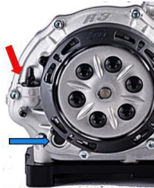
Figure 1: Location of the oil filler plug and the level sight glass
